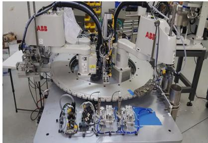
*Cobb Tool recently created a series of custom machined parts that serve as the nests and guides for an automated robotic assembly machine in the manufacture of complex electrical connectors.*
